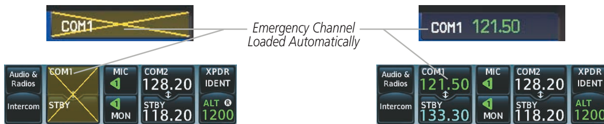
Figure 4-61 COM Tuning Failure
