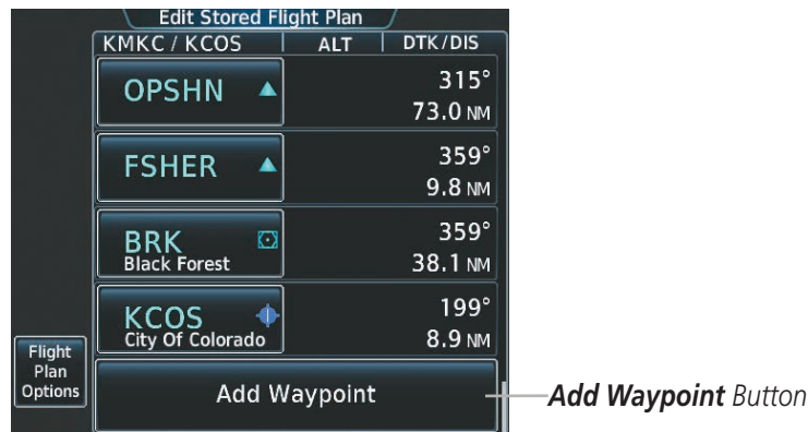
Figure 5-92 Edit Stored Flight Plan Screen - Adding a Waypoint to the end of the Flight Plan
