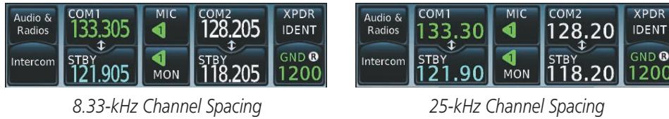
Figure 4-13 COM Channel Spacing
