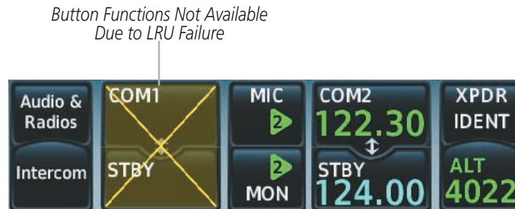
Figure 1-21 Failed Buttons on Touchscreen Controller
