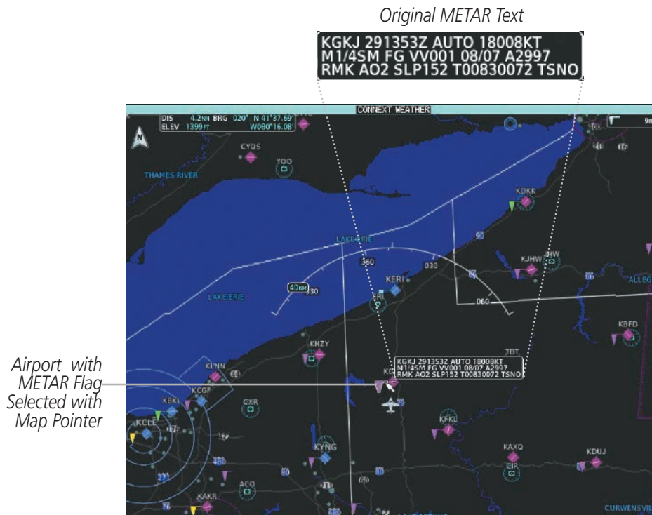
Figure 6-64 Viewing METARs on the Connex Weather Pane
