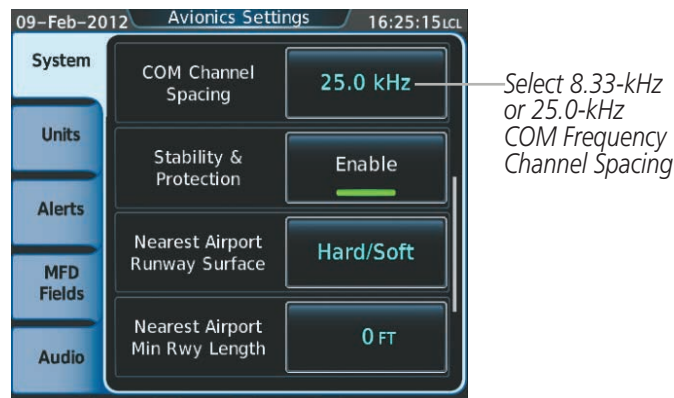
Figure 4-14 Changing COM Frequency Channel Spacing
